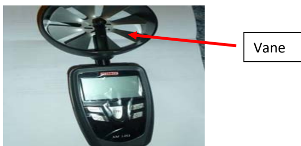
Figure 2: Example of a vane probe thermo anemometer
